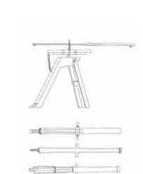
The weapons used in gunnery towers such as the Revellín Tower were small calibre and were mainly used to defend the moat alongside the walls.
